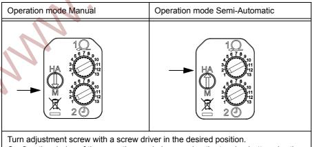
Confirm the choice of the operation mode by pressing the tension button shortly.
