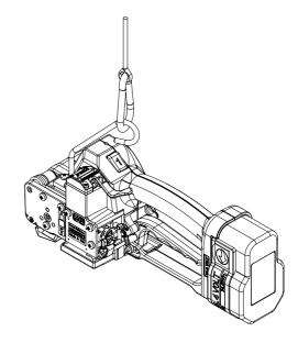
For working in alternating positions a turn able suspension bracket with screws and washers can be ordered under item number P32.0137.
