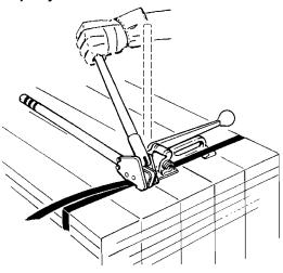
2. Bring sealer handles completely together to assure a proper notch.
