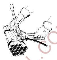
Notch the seal with a Signode sealer to complete the joint.
