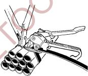
Break off the strap at the seal by repeatedly raising and lowering the tool. Inspect the joint to make sure the seal has been properly notched. Refer to the sealer Service Manual.
