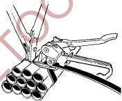
6. Break off the strap at the seal by repeatedly raising and lowering the tool. Inspect the joint to make sure the seal has been properly notched. Refer to the sealer Service Manual.
