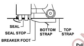
back on the TOP STRAP to eliminate additional slack around the package. You will have to push on the cylinder cover to make certain that the jaw tips are in position over the seal.
