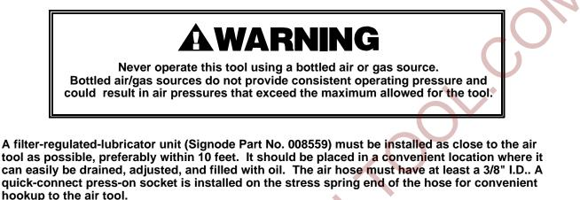
Filter and lubricator bowls are made of polycarbonate material. Do not install where bowls may be exposed to materials incompatible with poly carbonate. Certain oils, solvents, and chemicals or their fumes can weaken these bowls and possibly cause them to burst. Clean only with warm water. A cut-off valve placed ahead of the filter will be useful when cleaning the filter or replenishing the lubricator.
