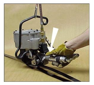
4. If strap alignment is unsatisfactory and it becomes necessary to shut off the tool during the tensioning portion of the cycle, push down on the stop lever.
