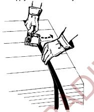
3. While standing to one side of the strap line, tension the strap through continuous up and down motions with the tensioning handle. NOTE: Do not allow the handle to press against the base during the downward portion of the tensioning cycle. This will raise the feedwheel and release the tensioned strap.
