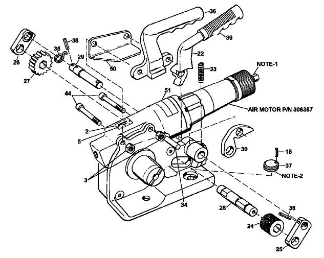
NOTE 1. Use large quick disconnect fittings: Socket P/N 0200706, Plug P/N 020704 NOTE 2. Assemble wear pad with "B" side down.
