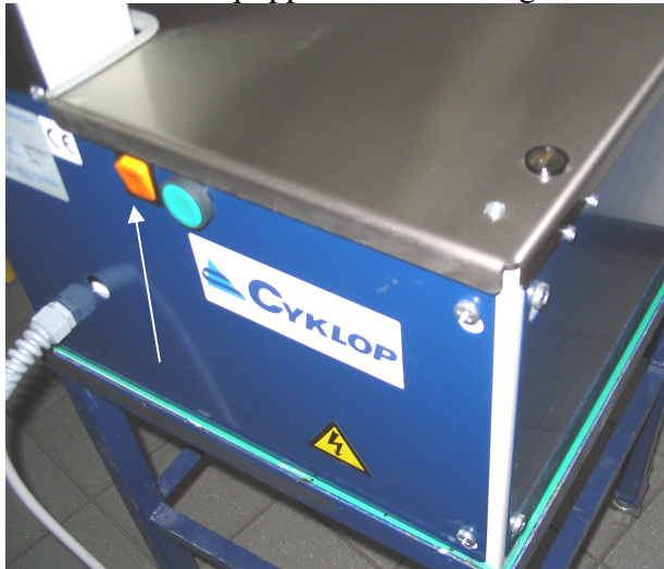
Figure 3: Mains switch used for the various versions
