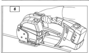
Opening and extraction of the tool. <u>Wait for weld to be cooled before extracting the tool. A count down on</u> the display and an acoustic sound signals the end of the cooling time. An anticipated opening of the tool could cause an excessive loss of tensioning force or break of the weld with consequent serious danger for the operator.
