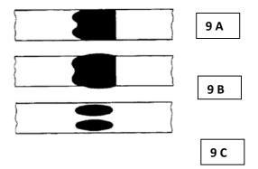
ATTENTION! <u>Cut and replace strappings with inadequate welds. Eventual break of the strap in the welding</u> area could cause serious damages. <u>Test, periodically, the effective welding efficiency with adequate</u> equipment (Strap samples can be sent to DuBose for testing and documentation).
