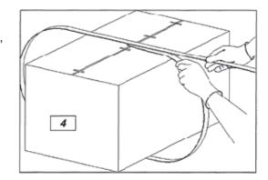
Strap insertion. With your right hand, open the tool raising the opening lever (fig. 5). With your left hand, insert both straps keeping them well aligned. Release the opening lever. Check the correct positioning of the straps before proceeding.
