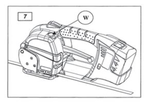
Opening and extraction of the tool. Wait for weld to be cooled before extracting the tool. A count down on the display and an acoustic sound signals the end of the cooling time. An anticipated opening of the tool could cause a excessive loss of tensioning force or break of the weld with consequent serious danger for the operator.
