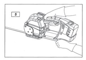
Start of the strapping cycle. Check the selected operating mode. Stay to the side to avoid eventual lash of the strap due to excessive tensioning force and consequent break of the strap. Press the tensioning button (1.1) see (fig.6). In both manual and semiautomatic modes the tensioning of the strap stops if the tensioning button is released. In automatic mode, the strapping cycle could be stopped at any moment by pressing the tensioning or welding buttons or raising the opening lever.
