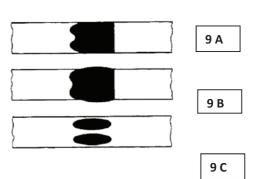
ATTENTION! Cut and replace strappings with inadequate welds. Eventual break of the strap in the welding area could cause serious damages. Test, periodically, the effective welding efficiency with adequate equipment (Strap samples can be sent to DuBose for testing and documentation).
