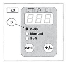
**Soft tensioning** – the soft tensioning can be applied on each of the basic operating modes: manual, semiautomatic and automatic. It consists in a lower speed tensioning and longer acceleration times in order to obtain lower tensioning forces. The soft tensioning is recommended where the package could be easily damaged and/or where a low tensioning force is requested. The soft tensioning is particularly suitable for a low thickness straps and/or PP straps.
