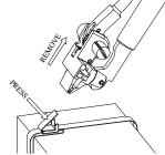
10. Hammer down wings securely using hammer knob on tensioner, or a similar tool.
