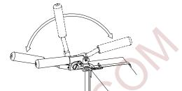
7. With strap tightened, bring tension lever back to original position, hold both handles together, and tilt forward as shown.
