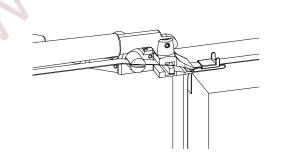
6. Holding the shear lever with the right hand, push the tension lever back and forth in a full arc with the left hand to tighten the strap.
