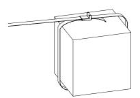
3. Bend back the lower layer of strap to form a hook around the bottom of the seal. Pull strap snug about package, with seal approximately one inch from the edge, as shown.
