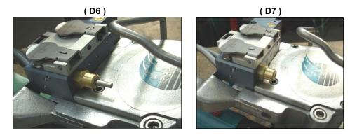
WARNING: Wait until the piston returns (pic.D7) before releasing the strap
