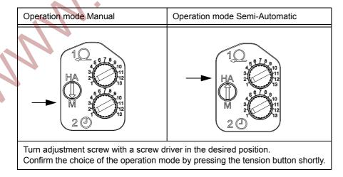
Adjusting knob tensioning force / tensioning speed Adjusting knob
