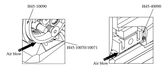
(2) If air gun could not dislodge the debris between the teeth of Tensioning Wheel (H45-10090), it is suggested to sharp the tip of PET (or other plastic) strap and use it as a tool to clean the strap debris.
